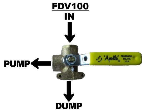
**HIGH LIFT 13MM MODEL 100 FLOW SCHEMATIC
